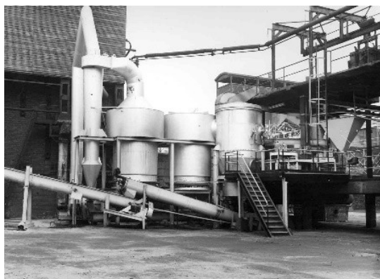
Experimental version of the fluid-bed roaster.
